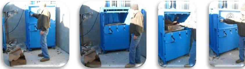
Close the door and push the handle all the way down. The baler will start automatically.
